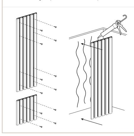
The Louvre Acoustic interior wall panels are designed to merge together to create a continuous, even wall surface of battens. Place a new panel on the tongue and groove at the edge of the previous panel.
